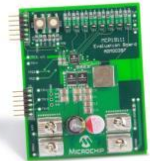
MCP19111 Evaluation Board (Part # ADM00397)
